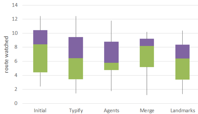
Figure 15: Box plot of the results for the number of times the route was watched in a trial. The participants watched the route more often with the INITIAL multi-scale map.
